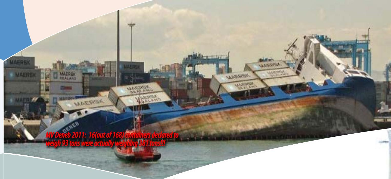
*MV Deneb 2011: 16(out of 168) containers declared to weigh 93 tons were actually weighing 381 tons!!!*
