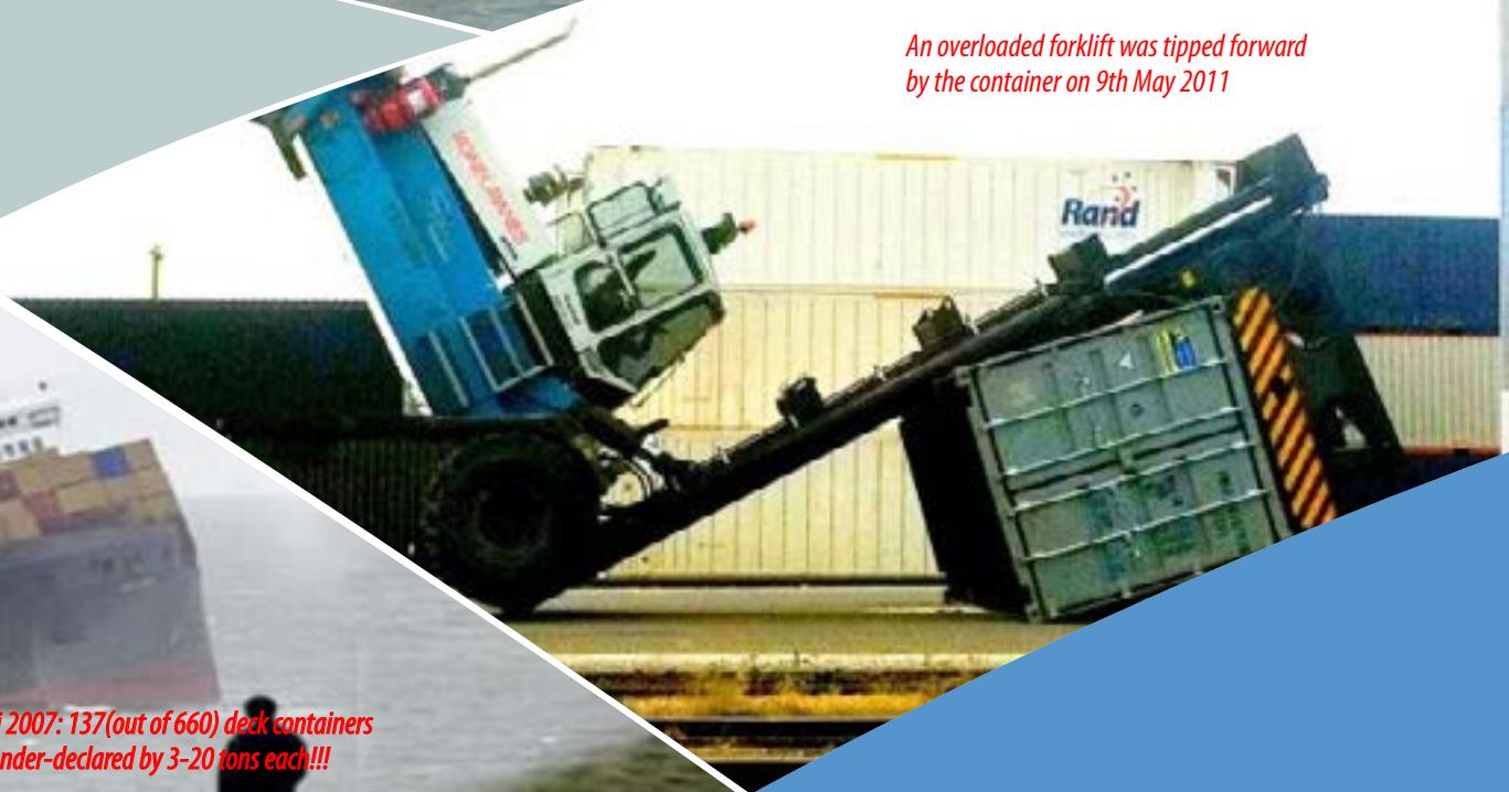
*An overloaded forklift was tipped forward by the container on 9th May 2011*
