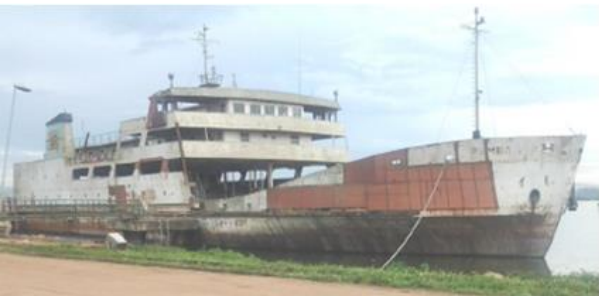
Above: NY Pamba, wagon ferry at Port Bell pending refurbishment. Below: Refurbished NY Kaawa, its operations on Lake Victoria have been inefficient largely due to the dysfunctional railway system; the wagon ferry is loaded and offloaded manually using human labor as opposed to driving off and on board loaded wagons onto the ferry at the ports of loading/offloading cargo. NY Kaawa and NY Pamba each has a capacity to carry 22 loaded wagons i.e. 44 TEU's.
