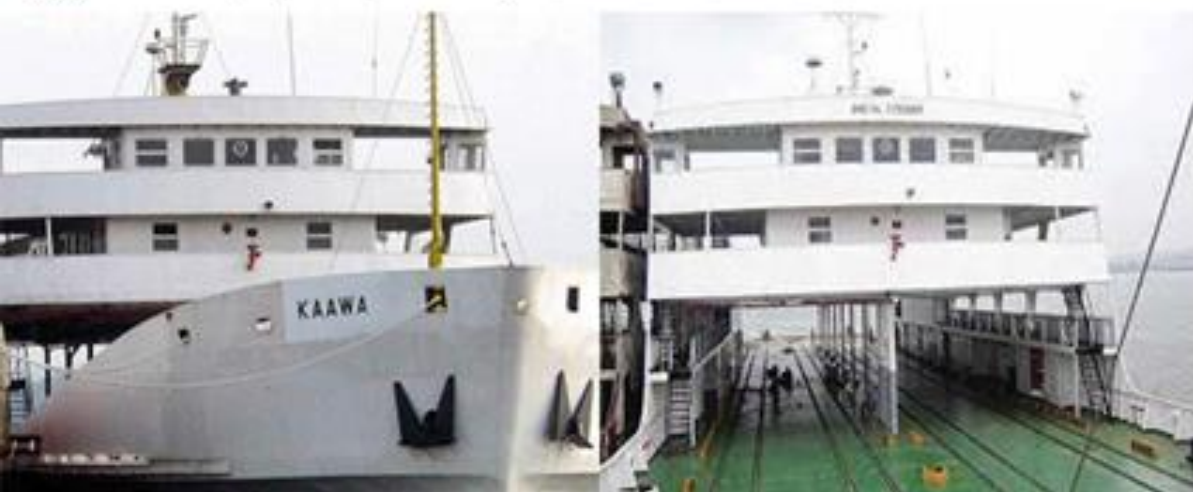
Above: NY Pamba, wagon ferry at Port Bell pending refurbishment. Below: Refurbished NY Kaawa, its operations on Lake Victoria have been inefficient largely due to the dysfunctional railway system; the wagon ferry is loaded and offloaded manually using human labor as opposed to driving off and on board loaded wagons onto the ferry at the ports of loading/offloading cargo. NY Kaawa and NY Pamba each has a capacity to carry 22 loaded wagons i.e. 44 TEU's.
