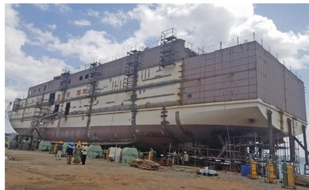
Figure 13: MV Mwanza under construction at a slipway in Mwanza South
