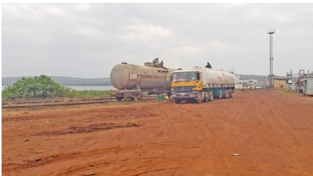
Figure 19: A truck drawing fuel from the wagon tank at Jinja Port due to lack of shunting locomotives
